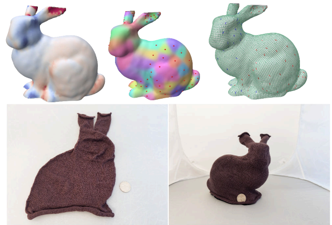
Fig. 16. Top. Left: Course curl signal. Middle: Power cells quantizing positive course curl. Right: Knit graph with left ends of short rows in red and right ends of short rows in blue. Bottom. Left: Knitted bunny without any stuffing or dressing. Right: We dress our knits on underlying 3D prints.
