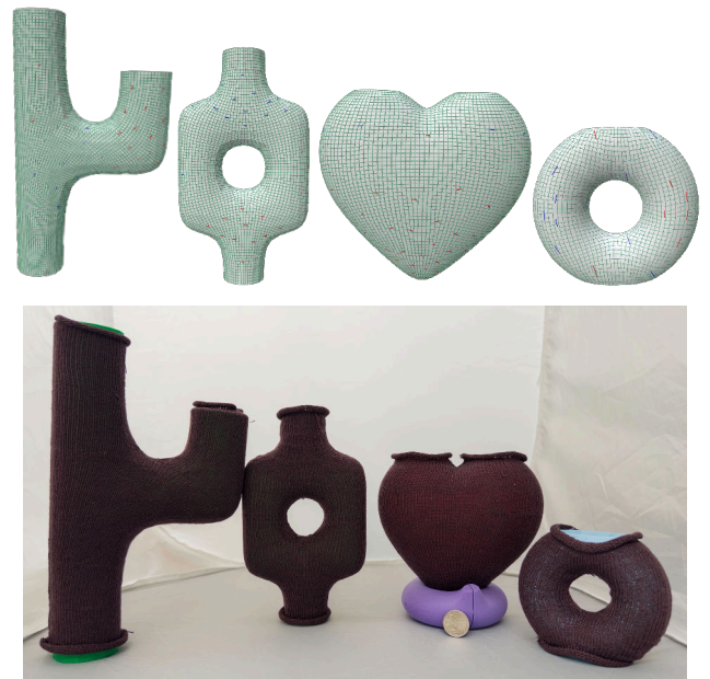
Fig. 17. From left to right: Cactus, pipes, heart, doughnut. Top row: Knit graphs highlighted with singularities. We show the short-rows on the cactus and doughnut models and the increases/decreases on the pipes and heart model. Bottom: Knitted results dressed on 3D print molds.
