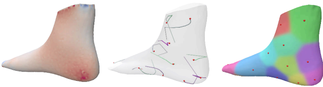
Fig. 7. Point trajectories on a sock model, starting from a random initialization. We quantize the positive portion of \nabla \times \nabla h (left) with a sparse number of singularities (12).
