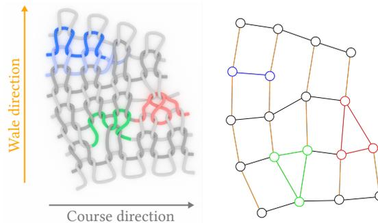
Fig. 1. A short row end, an increase, and a decrease, and the corresponding knit graph. Modified from [2].
