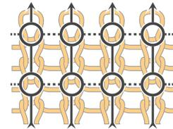
For areas without stitch irregularities, each node is part of four directed edges. Two are course edges, one incoming and one outgoing, and describe the overall direction in which yarn is laid down by the knitting machine. The other two are wale edges, one incoming and one outgoing, and describe the direction in which course rows are being produced.
