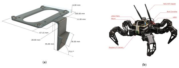
**Figure 3.** Hexapod physical augmentations and peripherals (a) CAD rendering of physical mounts for peripherals (b) modified PhantomX platform with Jetson Nano controller, Raspberry Pi Camera V2, buck convereter, U2D2, and Netis AC wireless adapter.
