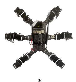
**Figure 1.** Trossen Robotics PhantomX hexapod (a) leg enumeration, rendered and simulated in ROS Gazebo (b) physical implementation of hexapod robot. For alternating tripod gaits odd enumerated legs move separately from even legs.
