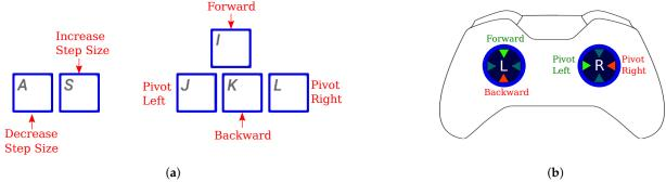
**Figure 9.** Evaluated operator interfaces to be compared against the proposed haptic interface **H** (**a**) keyboard layout for operator interface **K** (**b**) game controller mapping for operator interface **J**.
