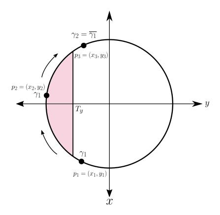
**Figure 6.** Pivoting phase is determined solely by transitions from outside to within the shaded region, determined by  $T_y$ . As the commanded position coordinates shift from  $p_1$  to  $p_2$ , the cursor enters the shaded region and the y position is less than  $T_y$ . When the cursor next leaves the shaded region, for example to  $p_3$ , the phases of the rotation is toggled, which alternates which set of three legs are raised.
