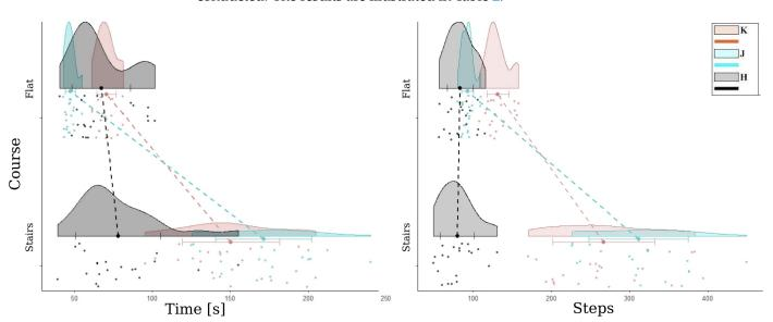
**Figure 13.** Performance robustness to increased task complexity. Left plot shows performance shift in time to completion, right shows performance shift for number of steps. Pink indicates **K**, blue indicates **J**, gray indicates **H**.
